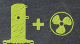
Fixed capacity compressor and single speed fan
